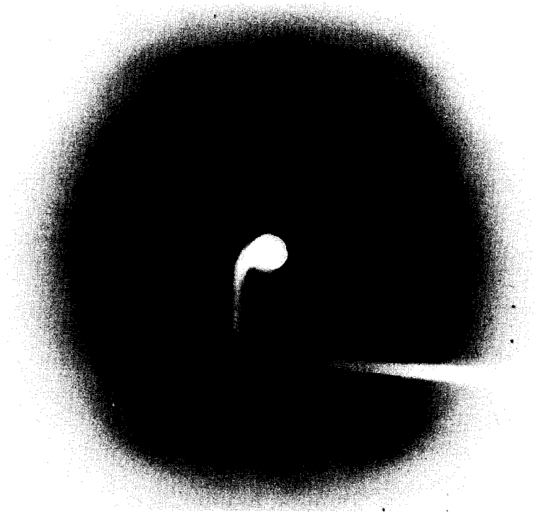
Figure 7 X-ray fibre diffraction pattern of the THF clathrate fibre annealed at 90°C (form I + form II)
